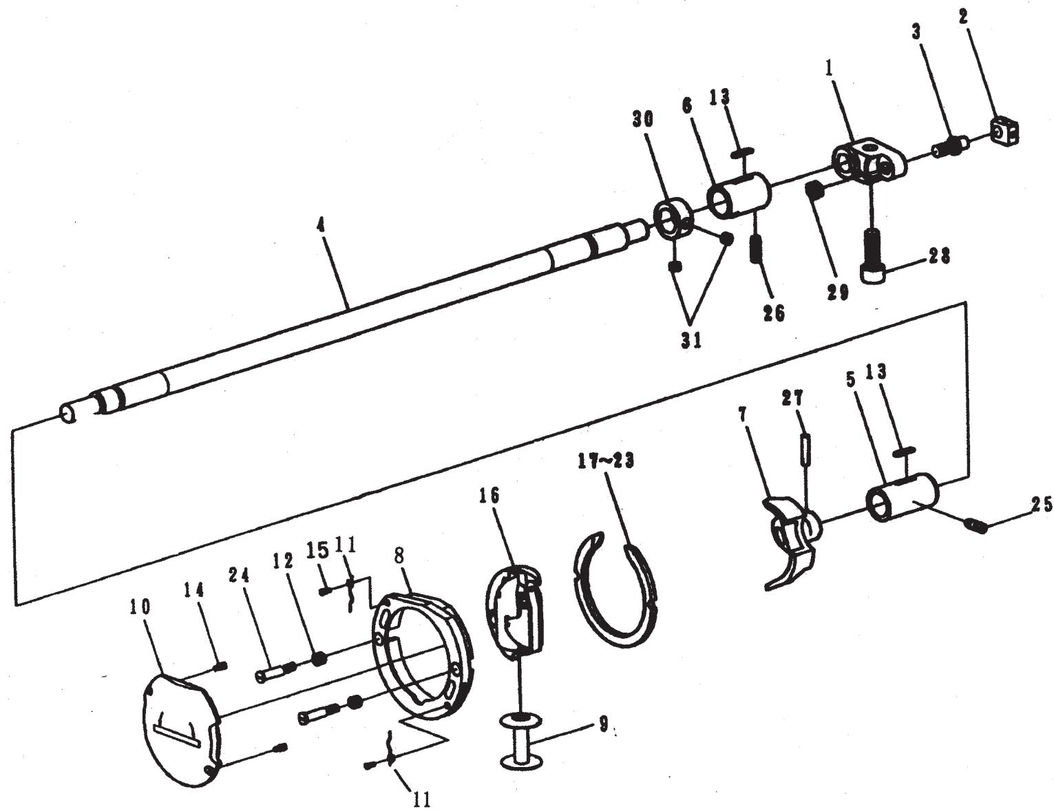
F. 下轴机构 HOOK DRIVING SHAFT COMPONENTS (1/2)
